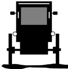
**This is the recommended way the side of a buggy should be illuminated.**
